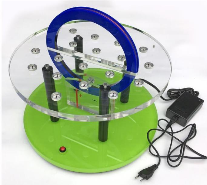
Pressing and holding a button to switch on an electric current through the coil produces a strong magnetic field, whose pattern is shown by the compass needles.
