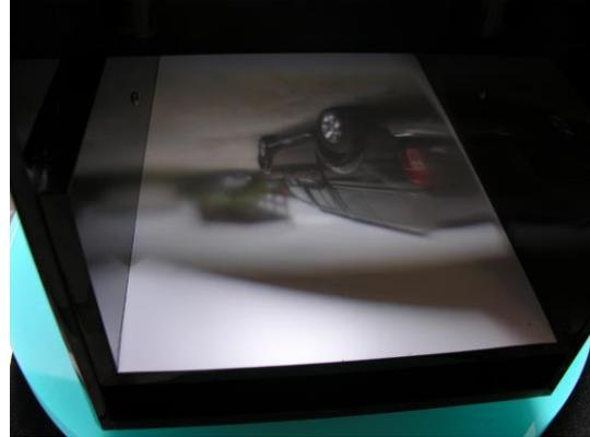
The mirror (which folds away for packing) reflects light downwards through a converging lens, forming an image on the horizontal screen inside the box. Using two red knobs, the screen can be raised and lowered to focus nearer or more distant objects. The whole unit can also be rotated on its base to 'scan' the view.
