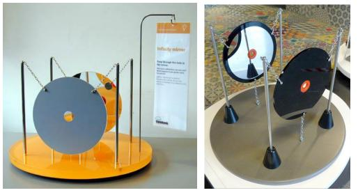
This is not an original idea, but provides plenty of scope for enjoyable experimentation. Each mirror has a central peep-hole giving an 'infinity tunnel' effect. Moving either mirror causes the 'tunnel' to 'bend'.
