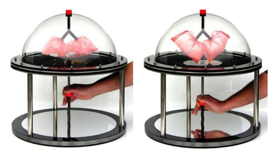
You pull down the red ball connected to a black rubber diaphragm. Air is drawn into the thin plastic bags through the Y-shaped tubes. If you put your finger over the top tube, you can feel the air flowing. It causes a 'wheezing' sound. The mirror underneath makes the red operating knob easily visible when the exhibit is displayed on a table of typical height.
