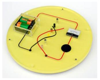
Two loose leads are used to find out which of the various material samples (plastics, metals, wood) allow current to pass through. Users are also prompted to search their pockets for more samples to test!
