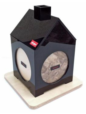
A simple model house with each of the four sides insulated differently: glass, stone, rockwool, polystyrene foam. An internal electrical lamp provides a source of heat. The different temperature of each outside wall can be measured with a separate thermal camera or an inexpensive infrared thermometer (not included).
