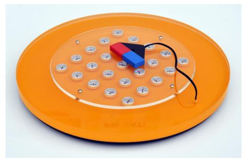
The compass needles are sensitive at a considerable distance from the coloured bar magnet and show the shape of the magnetic field.
