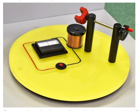
Can you make an electric current by moving the magnet near the coil? You will need to close the circuit, by pressing and holding either of the two red buttons. One of the buttons is connected to a small, black **diode** that only lets current flow in one direction. What difference does it make if you press and hold the other button?
