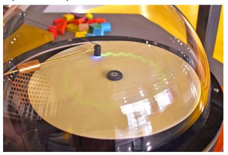
The LED draws a glowing line on the slowly rotating photophosphorescent plastic disc. The line fades within one rotation. The upper part of the exhibit is on flexible rubber mounts. When the 'hanging gate mechanism' is shaken, the LED draws a wiggly, line.
