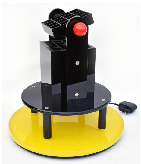
A balloon hovers above a low-voltage fan. Turbulence in the air stream is minimised by a 'straightener' unit above the fan. Turning the red knob adjusts the angle of a vane, deflecting the air flow and causing the balloon to hover to one side. A great crowd-puller!
