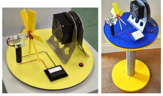
Like the simple version, but with an electrical generator, a meter with moving needle and a larger 50cm diameter base.
