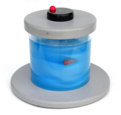
*Turn the handle to make the 'fish' swim round in either direction.* Notice the turbulent trail it leaves behind. Which swimming direction causes the least water disturbance?
